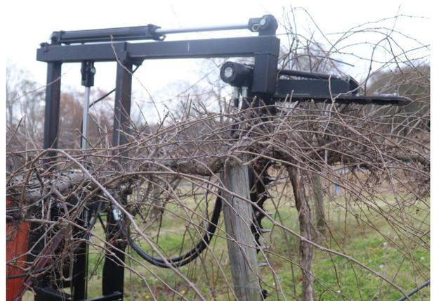
**Figure 2.** A tractor-mounted mechanical pruner in a dormant muscadine vineyard.
