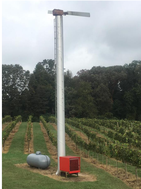
Figure 5. A wind machine in a young Chardonnay vineyard during the post-harvest period.
