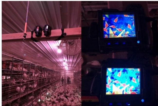
Figure 2. Thermal cameras setup above litter floor in the cage-free house.
