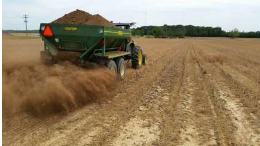
Poultry litter being spread on a cotton field using a small mechanical spreader. Photo credit: H. Tewolde [5].
