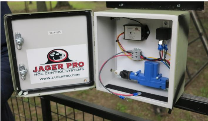
Figure 19. Remote controlled trap trigger.
