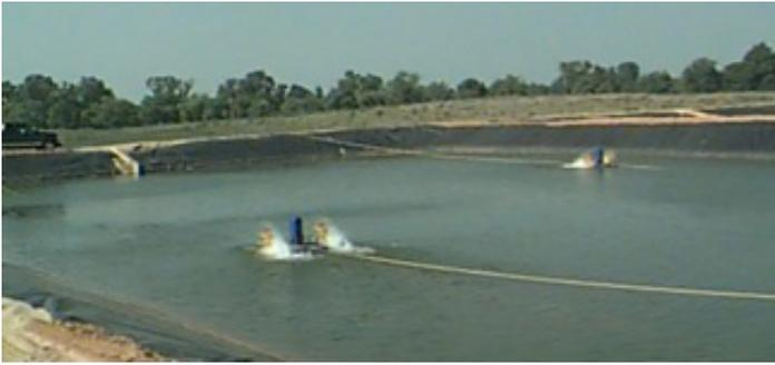
**Figure 3.** Paddlewheels are installed to create water circulation in ponds.
