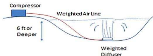
**Figure 2.** A compressor and diffuser system provides oxygen when bubbles diffuse into pond water.
