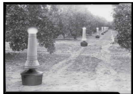
Figure 4. Return stack fuel oil heater in a citrus grove. Photo courtesy of USC Digital Library, D. Whittington Collection.
