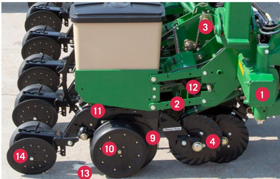
Always consult the operator's manual for the manufacturer-recommended settings for planter components such as vacuum, downforce, and closing wheel pressure to obtain optimal field performance. Properly lubricating all moving parts will help ensure efficient planter operation and extend the life of planter components.
