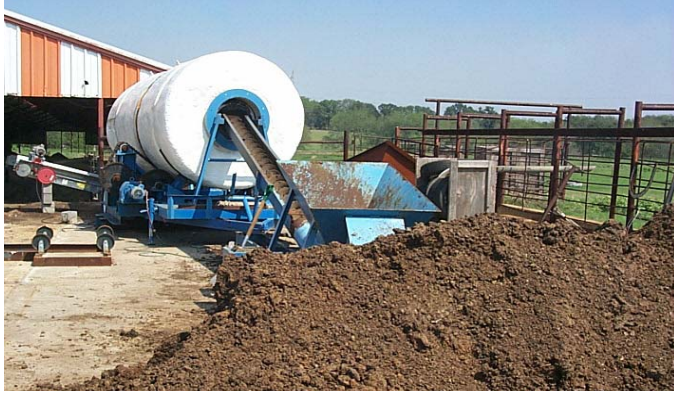
Figure 3.4-1 In-vessel composting system.
