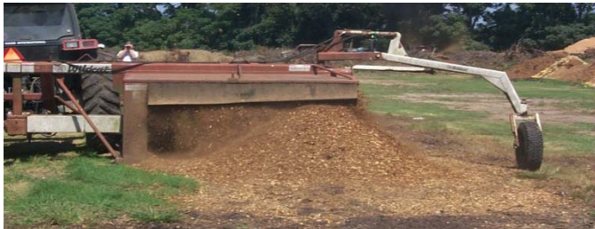
Figure 3.4-2 Tractor-driven windrow turner to aerate compost piles.
