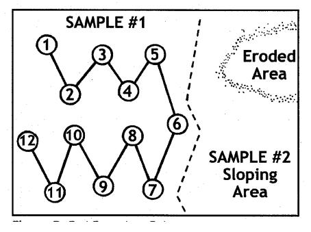
Figure 7. Zigzag pattern for collecting soil samples
