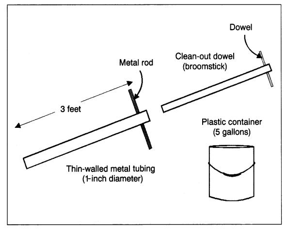
Figure 3. Solid manure sampling device
