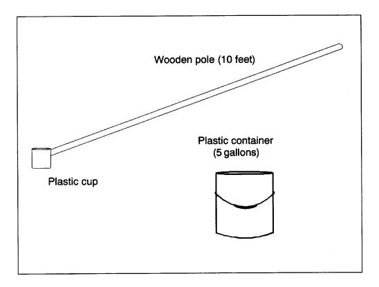
Figure 1. Liquid manure sampling device
