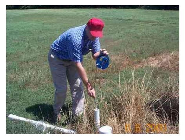
Figure 12. Measuring the depth to groundwater
