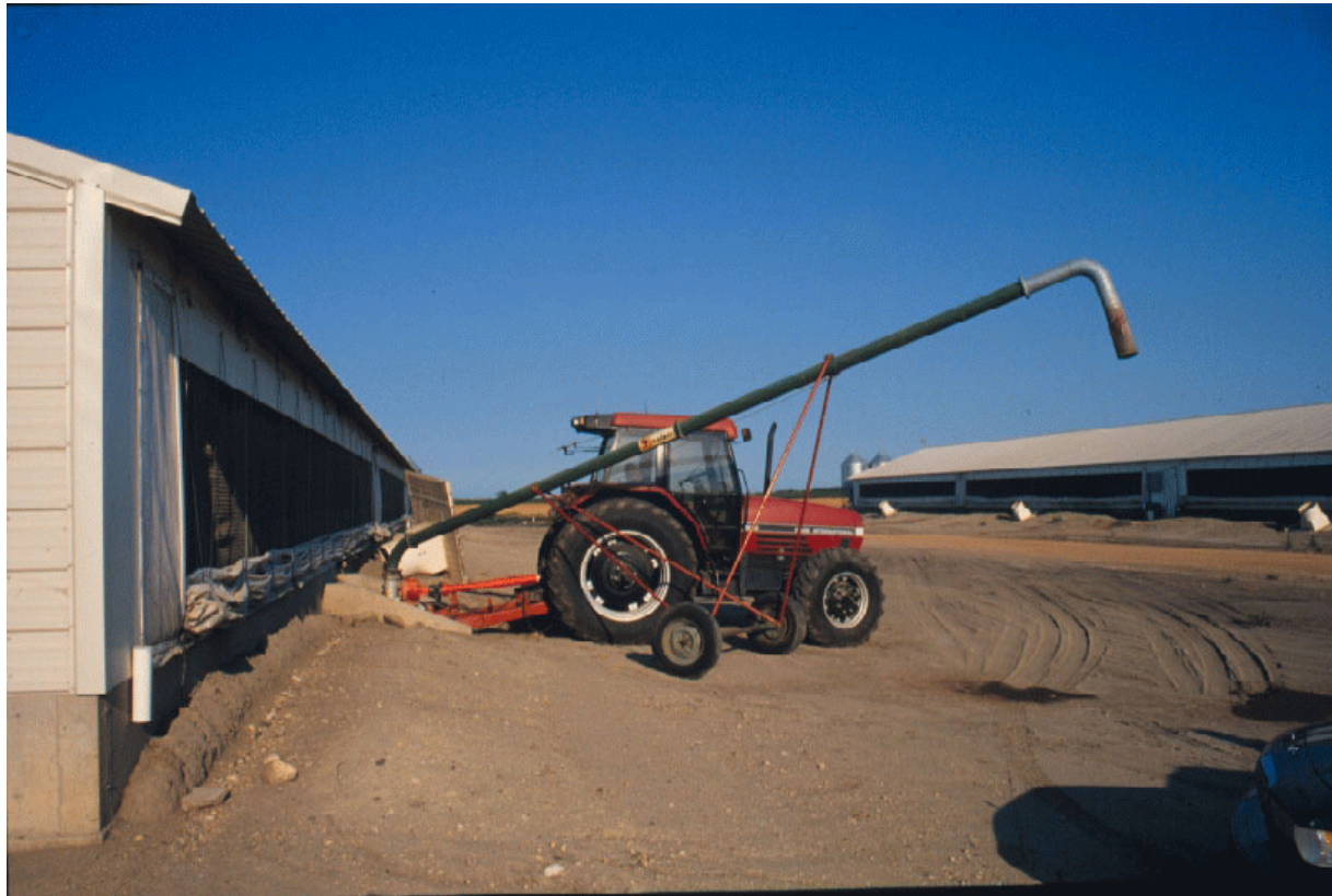
Figure 4. Agitation and pumping equipment for a deep pit manure storage under a pig-finishing barn.
