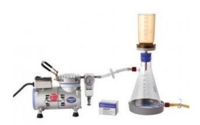
Figure 1. Total Suspended Solids (TSS) laboratory vacuum filtration unit. (Rocker Vacuum Filtration System, NewStar Environmental, Inc. – newstarenvironmental.com)
