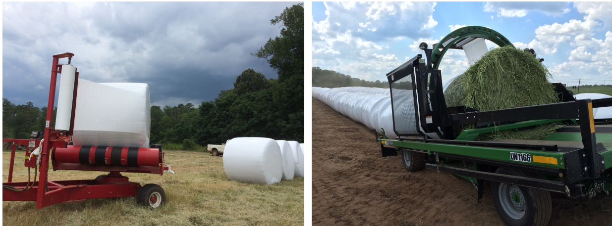
Figure 1. Examples of two basic categories of baleage wrappers: individual bale wrapper on a trailer platform (left) and an in-line bale wrapper (right).
