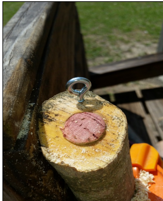
Cork hammered in; eye hook drilled in to hang trap.
